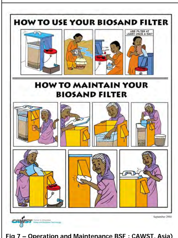
Fig 7 – Operation and Maintenance BSF : CAWST, Asia)
